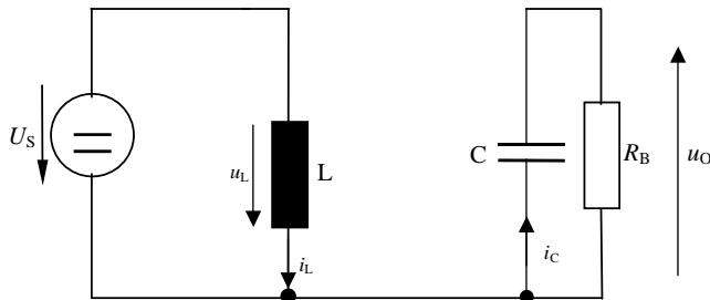
$$\Delta I_L(+) = \frac{U_s}{L} t_{ON} = \frac{U_s}{L} D T_s = I_{PK}$$
